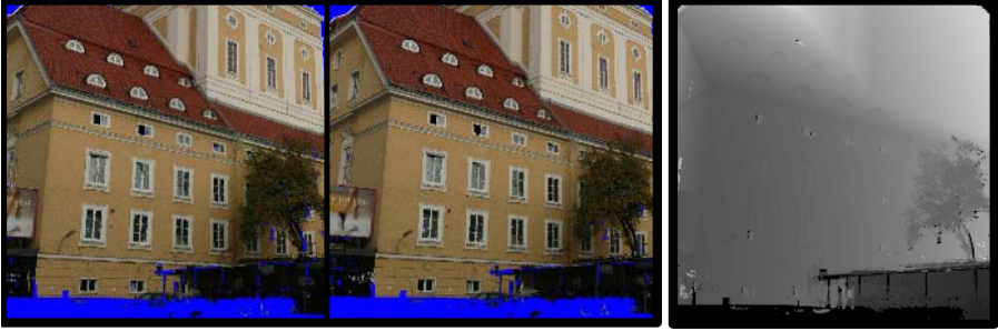
Fig. 4. Left and right image of one frame of the stereo image sequence (left) with 3D-ground truth (right)
