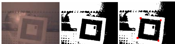
Fig. 2. Binarisation using dynamic threshold and corners detection: (from the left to the right) despite the darkness of the original image, it is possible to binarize it correctly and to detect pattern and its corners successfully
