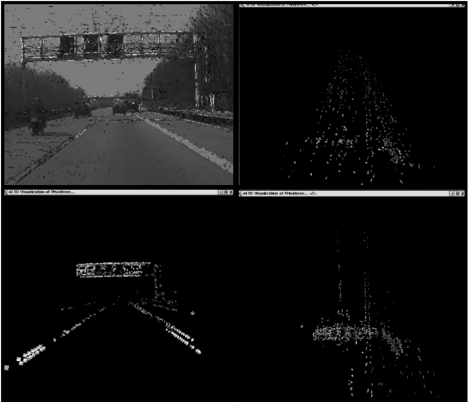
Fig. 6. Top row: Left: Confidences of different hypotheses are displayed by grey level values (white for high confidences and dark for low confidences) projected on the image. Right: Top view of the stereo of the first frame. Bottom row: Left: Image view of all hypotheses with high confidence after 5 iterations of the accumulation. Right: Top view of all hypotheses with high confidence after five iterations.
